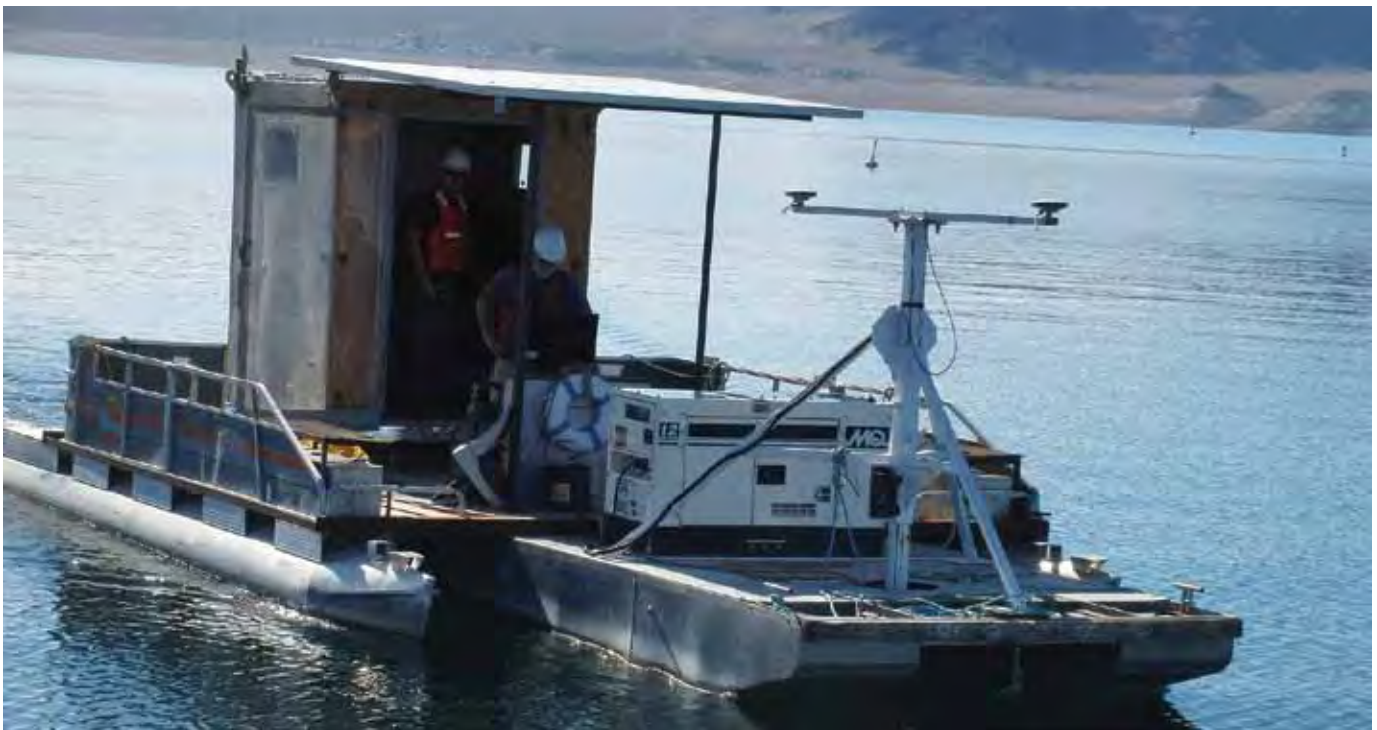
Figure 18. The survey boat with D-GPS antennas linked to a RTK-GPS on land, for georeferences capture of the underwater profile with the multibeam sonar.
