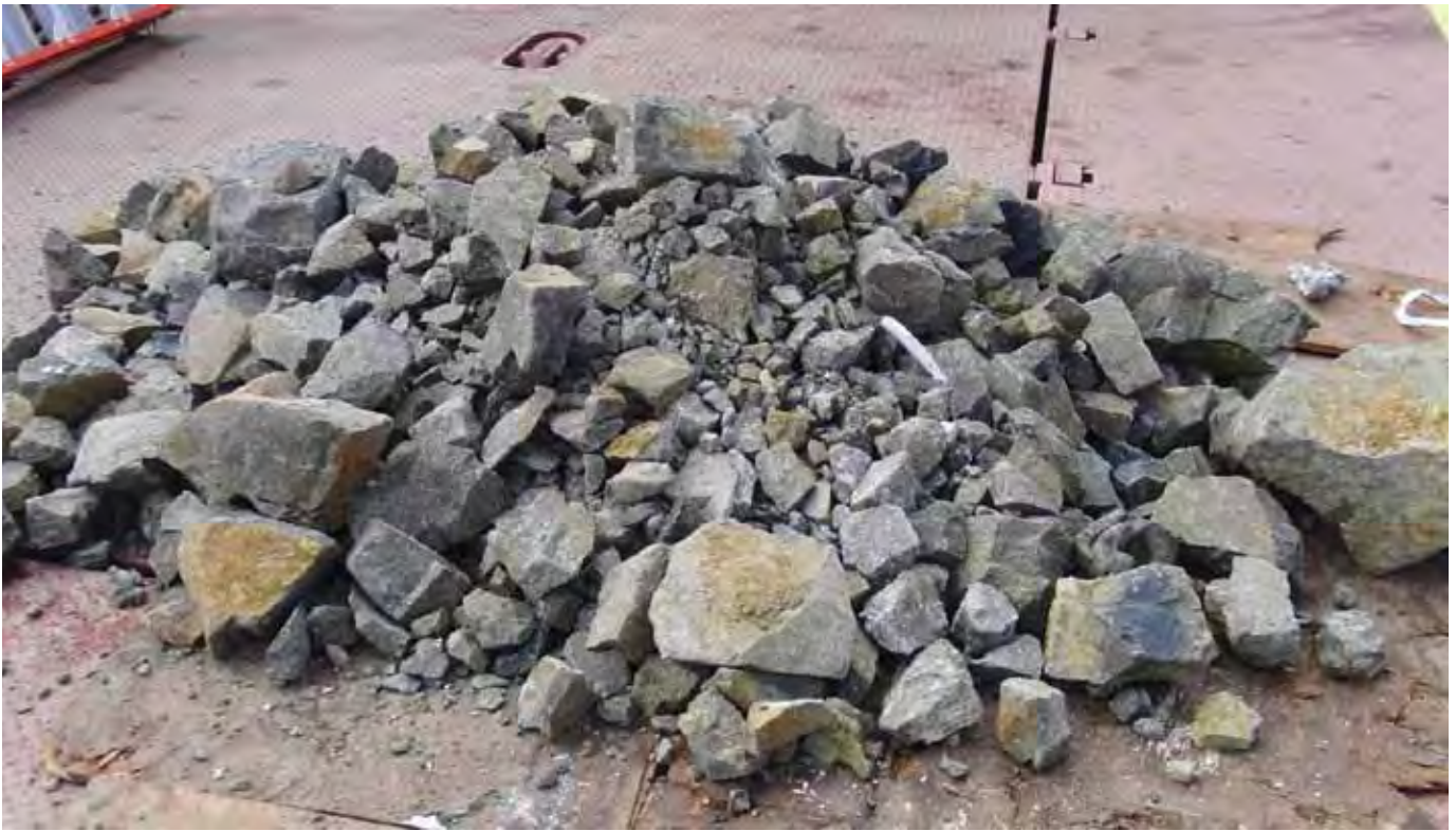
Figure 8. Broken rock mucked on the barge deck for sampling. Some old (brown) and new (gray) fractures could be noticed. The structure of the broken rock recalls that of the jointing seen in the open air outcrop on shore in Callville.
