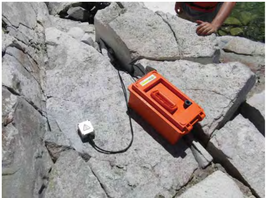
Figure 11 and 12. Blast induced vibration monitoring system and site decay curve.
